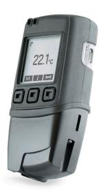
This standalone data logger measures and stores more than 250,000 temperature readings from a K, J or T-type thermocouple at a resolution of 0.1°C (0.2°F). It comes supplied with a K-type thermocouple capable of measuring from 0 to 200°C (32 to 392°F).
