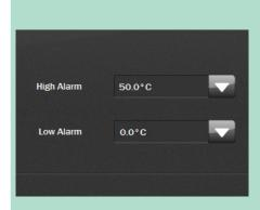
For each alarm that you have set, you must also set the level at which the alarm is triggered.
