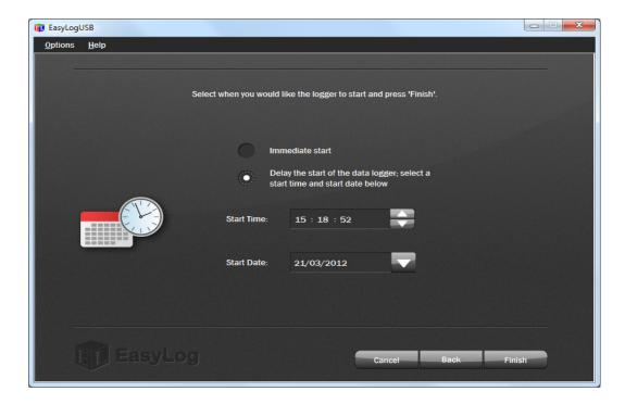
To delay the start of the data logger to a preset time and date, select that option and select the Start Time (hh:mm:ss format) and Start Date (dd/mm/yyyy format) at which you want to start logging, and click on the Finish button.
