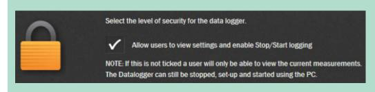
Some data loggers allow you to start, stop and then re-start data logging without the need for a PC.
