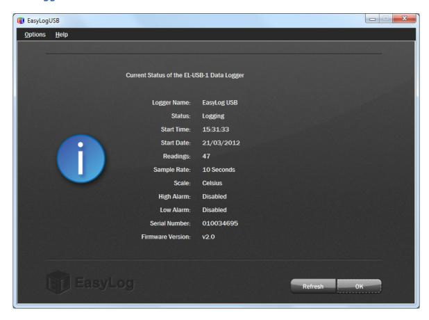
Click on Options > Current Status from the menu to display the current status of the attached data logger.
