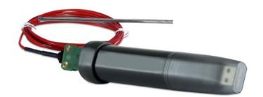
This standalone data logger measures and stores more than 32,000 temperature readings from a J, K or T-type thermocouple at a resolution of 0.5°C (1°F). It comes supplied with a K-type thermocouple capable of measuring from 0 to +200°C (-32 to +392°F).
