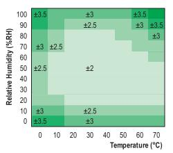
Typical and maximal tolerance at 25°C for relative humidity.
