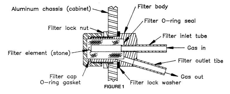
The stainless steel filter assembly is constructed as shown in Figure 1. It contains one replaceable filter element (stone) which must be thoroughly cleaned and dried, or changed every three months or 250 operating hours. The element is very simply removed and replaced in a few minutes from the outside of the gas generator, as follows:
