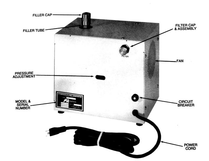
The Hydroflame III Soldering Unit requires only water and electricity for its operation. It produces hydrogen and oxygen at a controlled rate, automatically mixing them in the correct proportion for ideal combustion.
