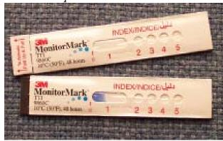
$3M^{\text{TM}} Monitor Mark^{\text{TM}} Time\ Temperature\ Indicators\ add\ an\ important\ temperature\ exposure\ measure\ that\ extends\ beyond\ your\ plant\ to\ your\ customers'\ delivery\ dock.$
