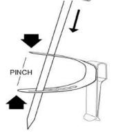
bottom of the holder. When the ends of the holder are released, the holder will expand to grab the probe securely. Use the clip to attach the holder to the side wall of a container. To remove the holder, pinch the ends of the holder and remove the probe.
