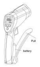
Locate the indentions on either side of the plastic case near the trigger. Open the battery compartment by pulling the rubber portion of the handle out and away from the trigger. Pull hard, it requires a good amount of force to open the battery compartment.
