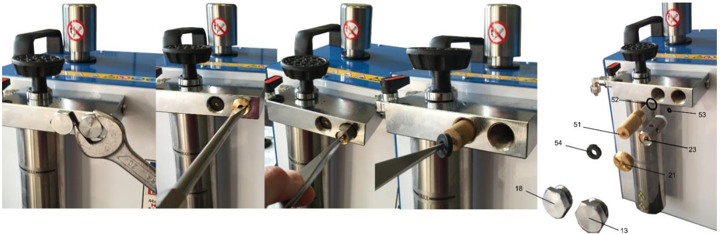
FIG 4 – CHECK VALVE AND BACK FLAME FILTER REPLACEMENT
