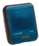
A standalone Alert Module for all the data loggers in the Diligence WiFi range. The Alert will pick up alarm messages from any Diligence WiFi data logger within WiFi range. It displays Red LED lights (through a Red translucent rear moulding) and sounds a substantial alarm (SPL 100dBA @1m) when a sensor alarm has been triggered. There are nine standard sounds to choose from.
